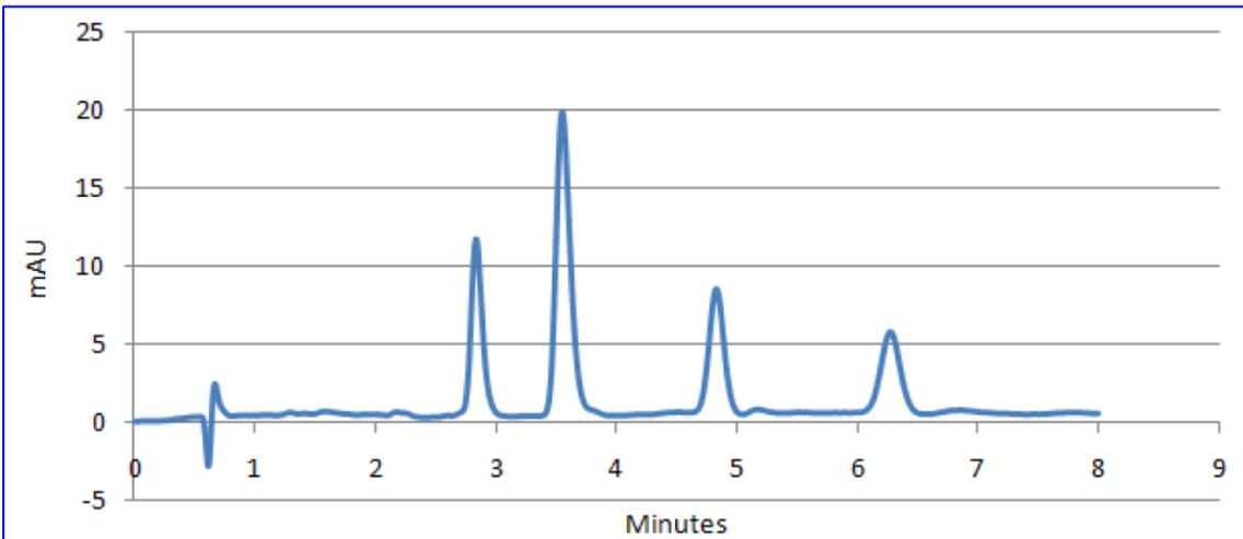
Figure 1. Standard 1 chromatogram showing the cohumulone peak at 2.8, the humulone/adhumulone peak at 3.7, the colupulone peak at 4.9, and the lupulone/adlupulone peak at 6.3.
